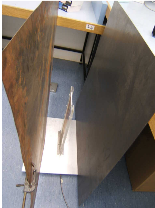
Figure 1.4: The triplate tapered slot element is paralleled with two metal sheets in the H-plane.
